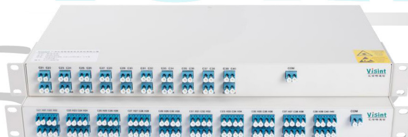
Figure 2: Integrated Multiplexing/Demultiplexing Equipment
