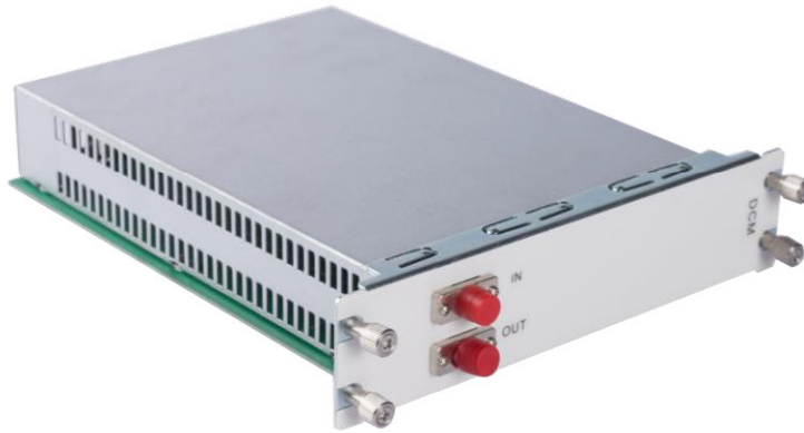
Figure 4: Fixed Dispersion Compensation Card (DCM)
