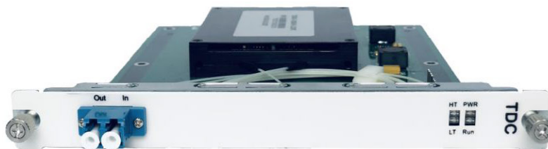
Figure 5: Tunable Dispersion Compensation Card (TDC)
